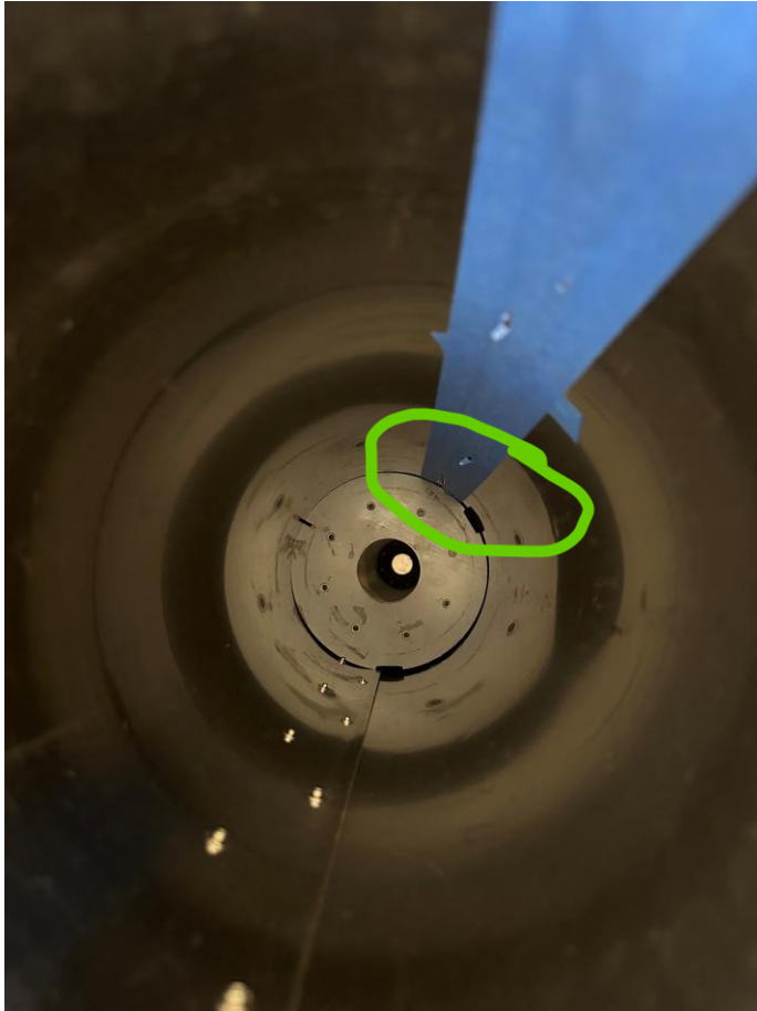
Degaussing Wire Damage
