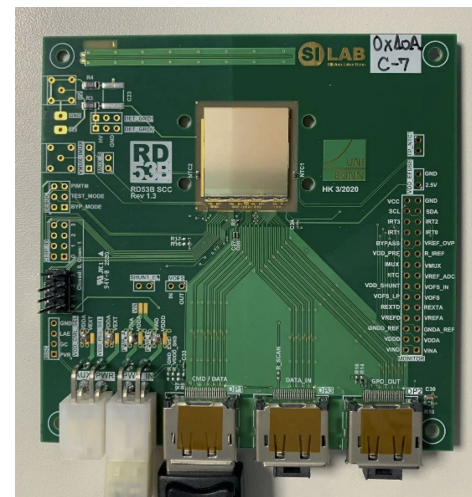
SCC (single chip card) used only for testing
