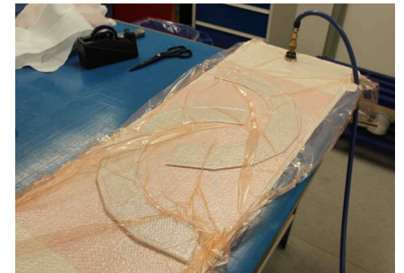
Vacuum-bagged co-cures (L3)
