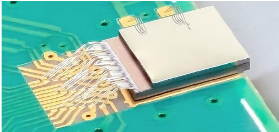
CLICpix2 bump-bonded to Si sensor
