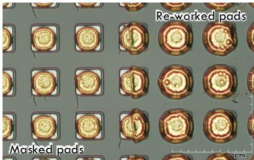
Timepix3 sensor after re-work
