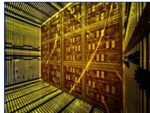
Construction of precision wire readout planes for the Short-Baseline Near Detector (SBND)
