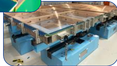
Construction of precision wire readout planes for the Short-Baseline Near Detector (SBND)
