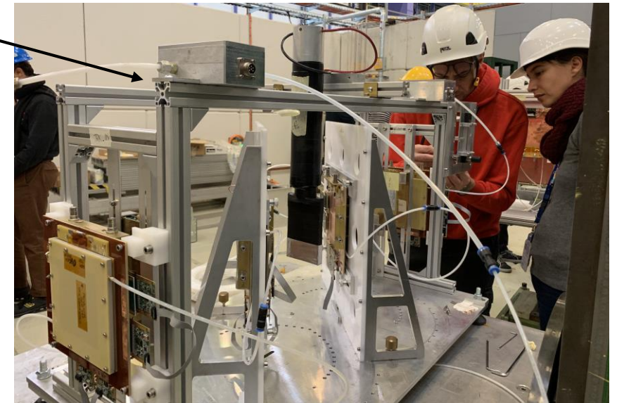
Detectors Under Test may be rotated to study resolution dependence for inclined tracks
