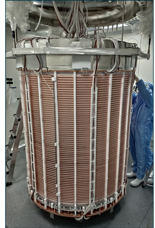
XENONnT: Drift field = 23 V/cm, Cathode = 2.75 kV
