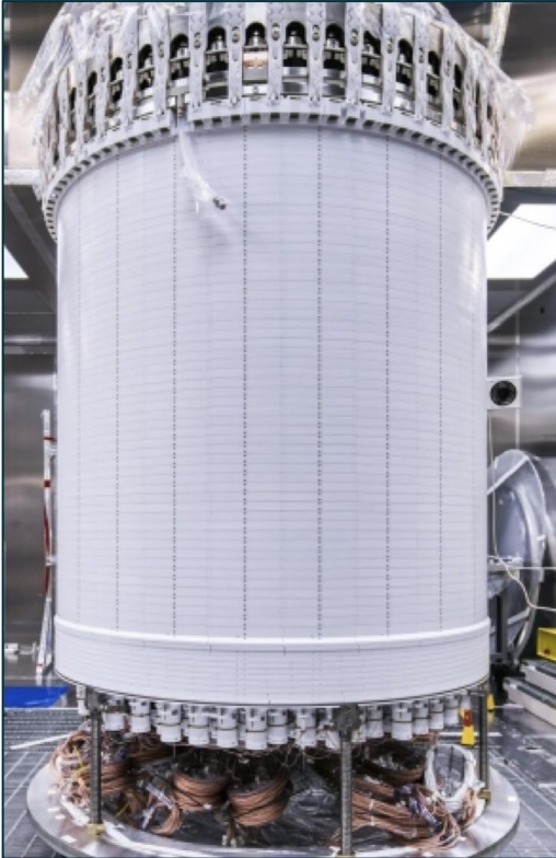
LZ: Drift field = 97 V/cm, Cathode = 18 kV
