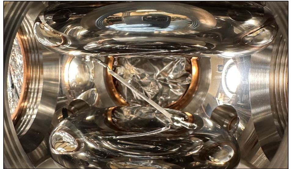
XeBrA electrodes with tapped threaded holes and resistor in place.
