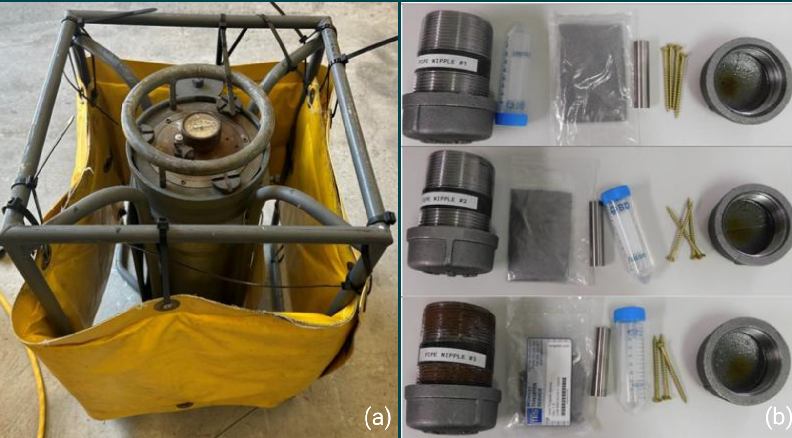
Figure 9: (a) The inside of the test waste drum is shown. The criticality cage holds the inner vessel and is surrounded by a lead blanket. (b) The inner vessel contains three pipe nipples with varying materials, including a bag of tungsten shot, a tungsten rod, a vial of water, and wood screws.
